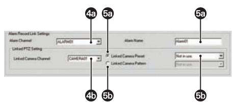
Figure 108. Event-PTZ Link Settings: Linking Presets and Patterns to Alarm Events
